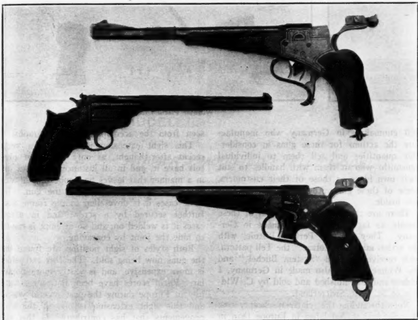
Top—Hartmann; Middle—S. & W.; Bottom—Widmer. Note Double Set Triggers on Hartmann and Side Lever for Operating Set Trigger on Widmer
